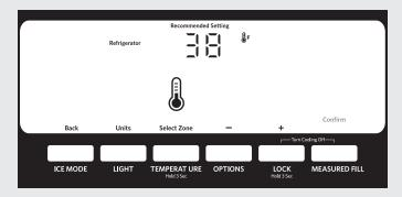
**NOTE:** To view Celsius temperatures, press the LIGHT button when adjust mode is activated. To return the display setting to Fahrenheit, press LIGHT again.
